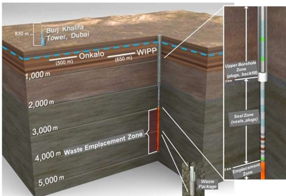
Fig. 1. Generalized schematic of the deep borehole disposal concept.
